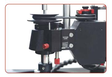
The O-ring drive is better suited for preparing delicate unencapsulated materials typically associated with TEM wedge thinning. The O-ring is able to absorb subtle resistive movements that could otherwise cause material fractures.
